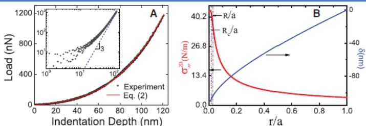
**Fig. 2.** (A) Loading/unloading curve and curve fitting to Eq. 2. The curve approaches cubic behavior at high loads (inset). (B) Maximum stress and deflection of graphene membrane versus normalized radial distance at maximum loading (simulation based on nonlinear elastic behavior in Eq. 1). The dashed lines indicate the tip radius  $R$  and contact radius  $R_c$ .
