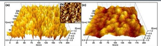
FIG. 3 (color online). (a), (b) 3D and 2D constant current STM image of monolayer graphene (1 V, 207 pA). (c) 3D tapping mode AFM image of the SiO<sub>2</sub> substrate (resonance frequency 326.4 kHz, force constant 47 N/m, excitation frequency 326.5 kHz, oscillation amplitude 18 nm, constant amplitude feedback, set point 90%). Note the identical scale of both images.
