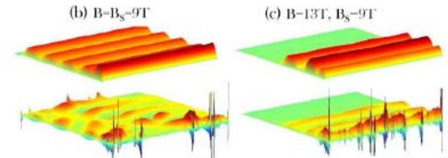
FIG. 6: (a) shows the conductance as a function of real magnetic field and Fermi energy, calculated for non-disordered zigzag ribbon with a strain geometry corresponding to  $W/R = 5$ , which is equivalent to  $B_s \approx 9T$ . (b) plots the current density at  $\epsilon_f = 0.1$  eV for the condition  $B = B_s = 9T$ , for perfect edge (top) and disorder edges (bottom). Similar plots for (c), except now for the condition of  $B = 13T$  and  $B_s = 9T$ .
