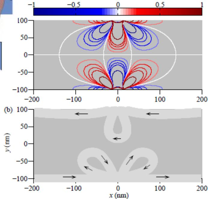
FIG. 3. (Color online). (a) Pseudomagnetic field, in Tesla, induced by two stamps with parameters  $2l = 30$  nm,  $c_0 = 1$  in a sample of width 200 nm. (b) Effect of this pseudomagnetic field on the edge states of the  $N = 2$  Landau level at  $B = 1$  T. The edge states are depicted as light gray ribbons of thickness  $l \approx 26$  nm. The arrows indicate their propagation direction.
