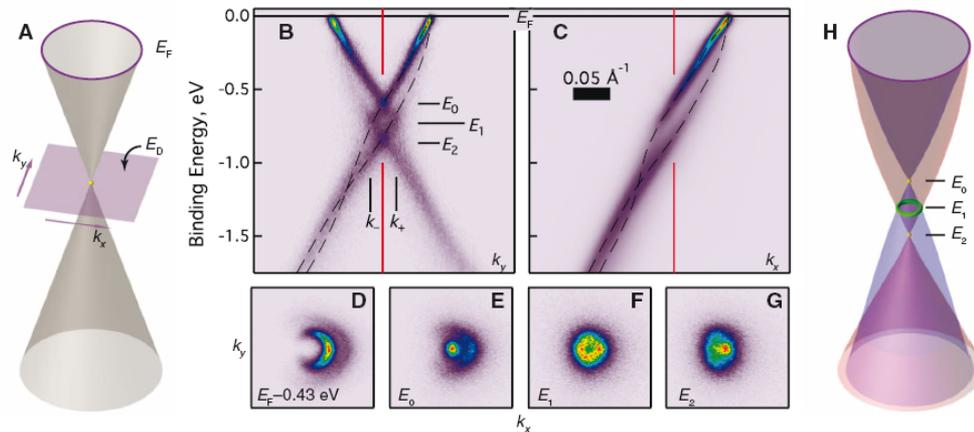
**Fig. 1.** (A) The Dirac energy spectrum of graphene in a non-interacting, single-particle picture. (B and C) Experimental spectral functions of doped graphene perpendicular and parallel to the  $\Gamma$ K direction of the graphene Brillouin zone. The dashed lines are guides to the dispersion of the observed hole and plasmaron bands. The red lines are at  $k = 0$  (the K point of the
