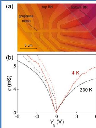
Two graphene layers separated by BN
