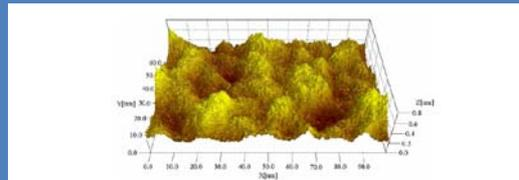
Fig. 3. Nanograph plot of a large-scale ( $100 \times 62$  nm) STM image of a single-layer graphene film on the silicon dioxide surface. The STM scanning conditions were  $V_{bias} = 1$  V (sample potential) and  $I = 0.5$  nA. The 0.8 nm scale of the vertical (Z) coordinate is greatly enlarged to accentuate the surface corrugations.
