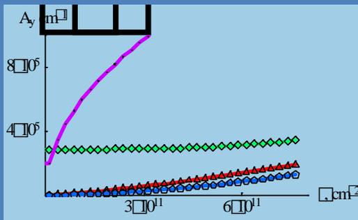
Vector potential inside the suspended region as function of carrier density for different values of the slack
