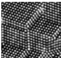
Atoms of silicon spacing ~tenths of nm
