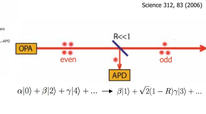
Single-photon subtraction from a pulsed squeezed state
