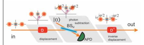
FIG. 1. (Color online) Schematic representation of the singlemode PHASE gate. BS stands for a mostly transmitting strongly unbalanced beam splitter, APD stands for avalanche photodiode, and D represents the displacement operation.
