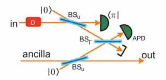
FIG. 4. (Color online) Schematic representation of the approximate single-mode Hadamard gate.  $BS_u$  stands for a highly unbalanced weakly reflecting beam splitter, while  $BS_{\Gamma}$  is a beam splitter with transmission coefficient  $t_{\Gamma}$  used to set the parameter  $\Gamma$ . APD stands for a avalanche photodiode and  $\langle \pi |$  represents the suitable projective measurement (see text).
